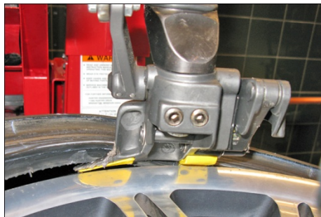
MOUNT HEAD CORRECTLY PLACED
