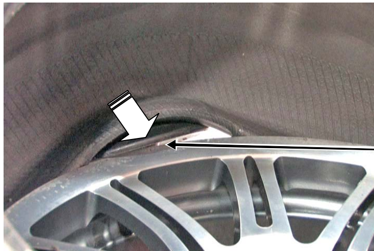
DISC REPOSITIONED AND LOCKED IN PLACE
