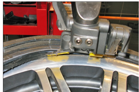
MOUNT HEAD INCORRECTLY PLACED
